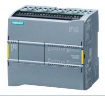
SIMATIC S7-1200F, CPU 1214 FC, compact CPU, DC/DC/relay, onboard I/O: 14 DI 24 V DC; 10 DO relay 2 A; 2 AI 0-10 V DC, power supply: DC 20.4-28.8 V DC, program/data memory 200 KB
